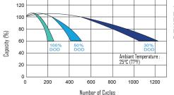
Testing condition Discharging:current D.17C A(FV1.7V/cell); Charging:current D.25C max, voltage 2.45V/cell; Charging volume:125% of discharged capacity.
